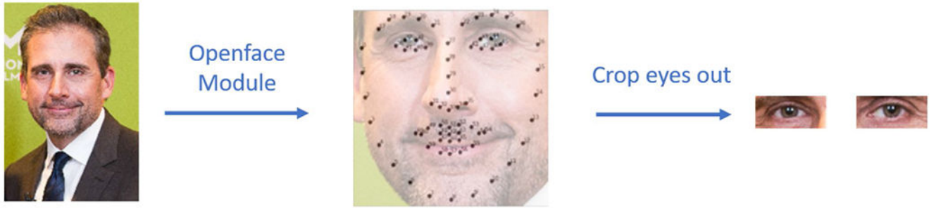
Fig. 2. Automated extraction of single eye images from a full-face photo using the OpenFace package. Key facial landmarks were identified (black dots in the center image) and then used to crop each eye for further evaluation.
