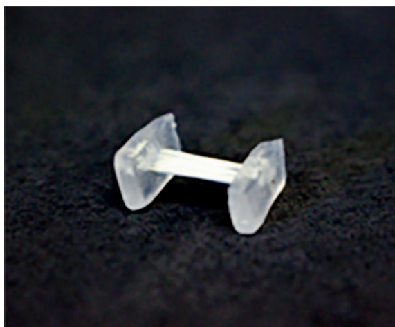
Figure 3. (a) Seven segments tightly arranged and fixed with transparent wax at both ends. (b) The measurement was conducted with a colorimeter using a shade tab.
