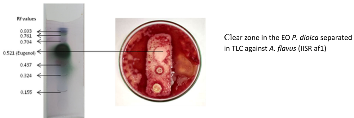
Fig. 4 Thin layer chromatography with agar overlay assay of the EO of P. dioica leaf against A. flavus (IISRaf1)
