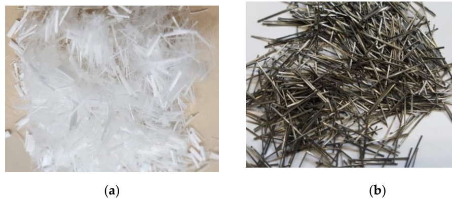
Figure 3. Types of fibres used; (a) PF and (b) SF.
