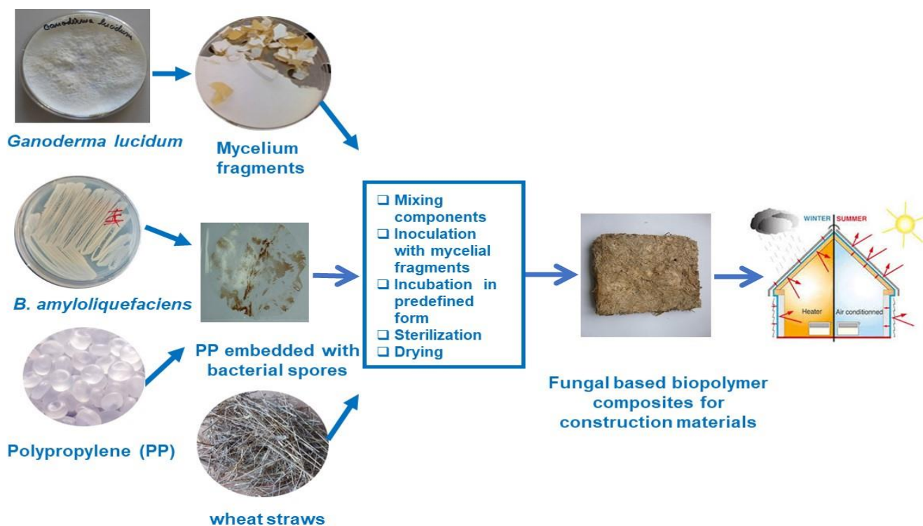
Figure 4. Schematic representation for preparation of fungal composite material.
