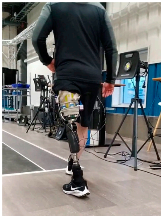
Figure 23. The prototype sensing system on a transfemoral amputee during the initial pilot trial.
