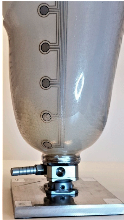
Figure 17. A QTSS™ pressure sensor inside a socket.
