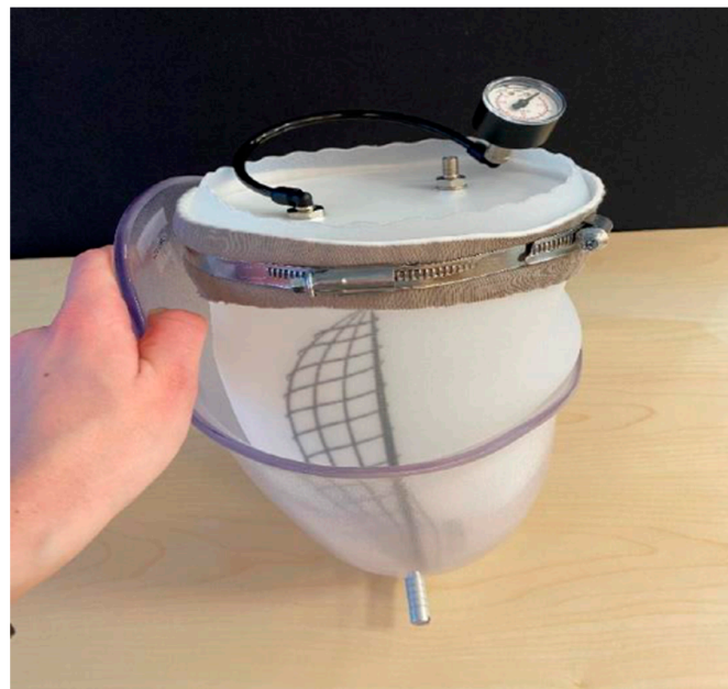
Figure 14. The liner balloon with a top plate.
