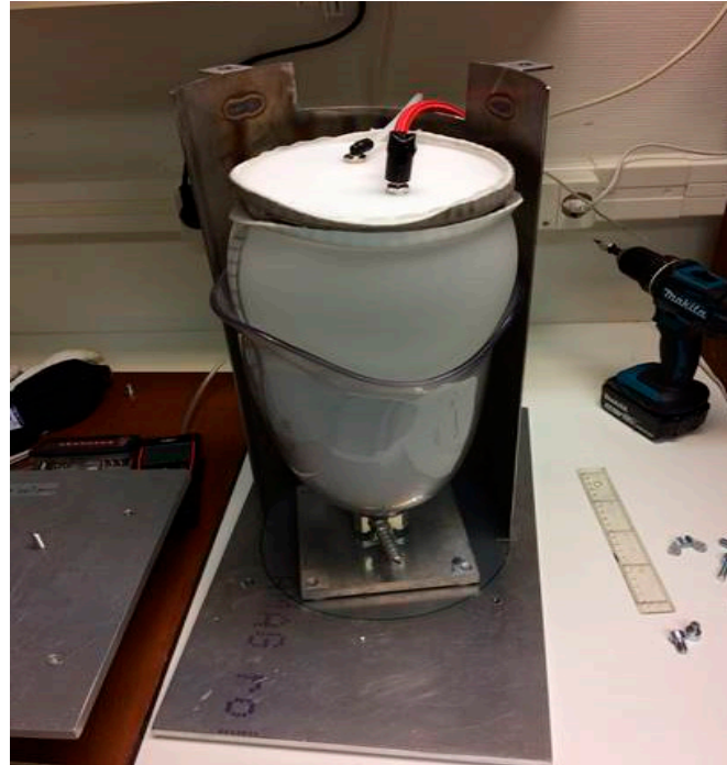
Figure 15. The liner balloon test setup on the base.
