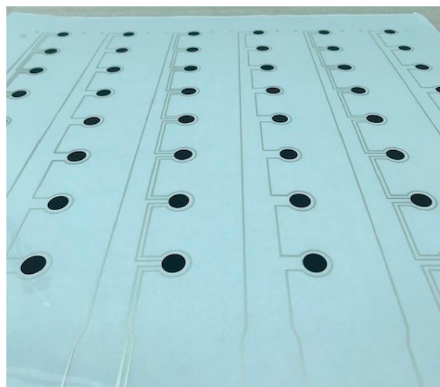
Figure 5. PET sheet screen-printed with multiples of the QTSS™ prototype pressure sensor strip design.
