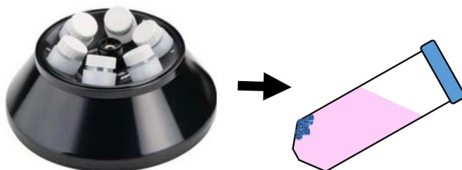
Figure 2. Position of pelleted viruses in centrifugation tubes after LSC. When using a fixed-angle rotor, the pelleted virus will appear as a clear, transparent pellet (blue dots) on the upper wall of the conical tube.
