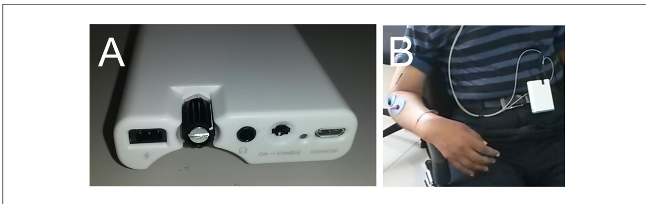
Figure 2. The experimental device: A. Photograph of the device, showing (from left to right) the connector for stimulating electrodes, knob for adjusting stimulus intensity, audio output to earpiece, switch to select between “on” and “charge,” LED to indicate when battery is fully charged, and micro-USB connector for charger. B. Device in use by a stroke patient in Kolkata as part of the trial to improve hand function.
