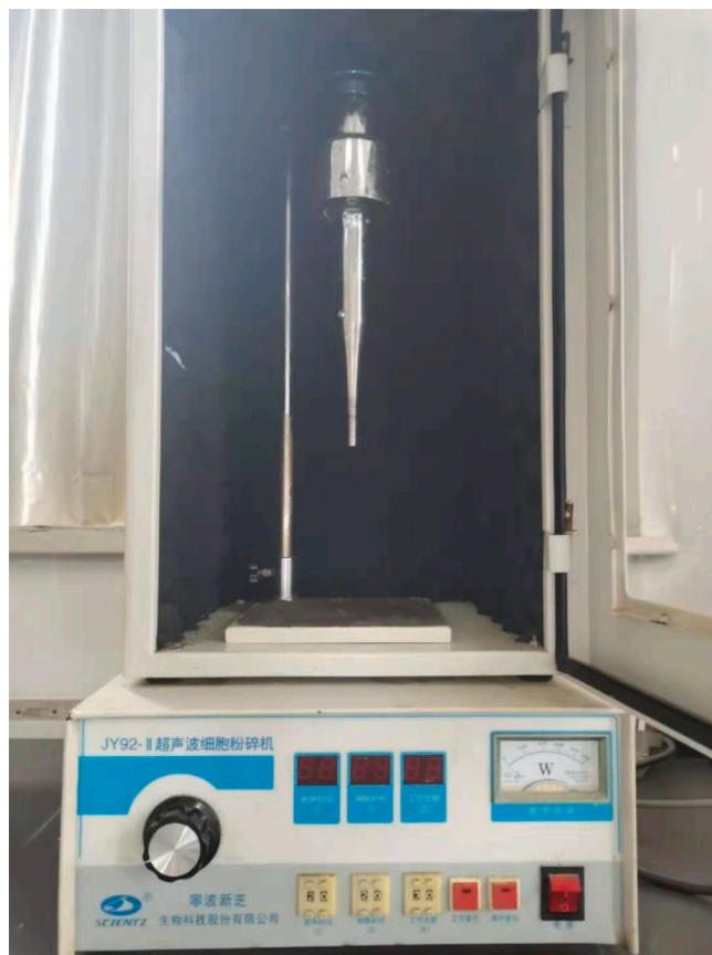
Fig. 4. Ultrasonic cell crusher used in this experiment.
