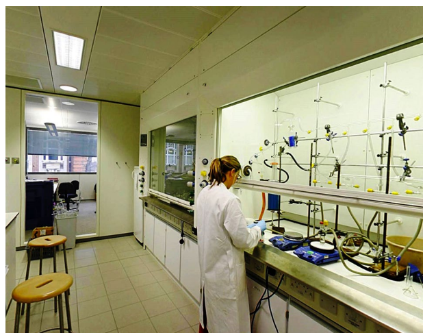
Fig. 14 Fume cupboard in the laboratory. The writing area can be seen outside, Chemistry Research Laboratory, Oxford, 2004. Photograph by Karl Harrison, © University of Oxford
