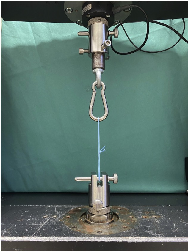
Fig 2. In the mechanical study part, each suture or tape loop construct was placed between a hook and a pin secured to the crosshead and base of the material testing machine.
