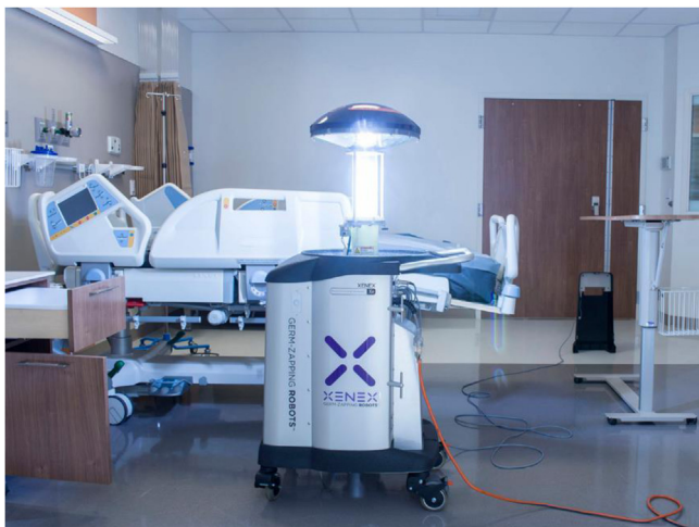
Fig. 2 – Ultra-violet robots are used for sterilizing purposes. Source: Xenex Disinfection services.
