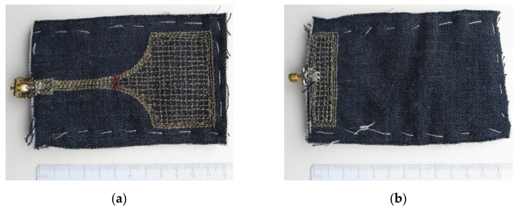
Figure 4. Wideband textile planar monopole: (a) radiating element and (b) ground plane.
