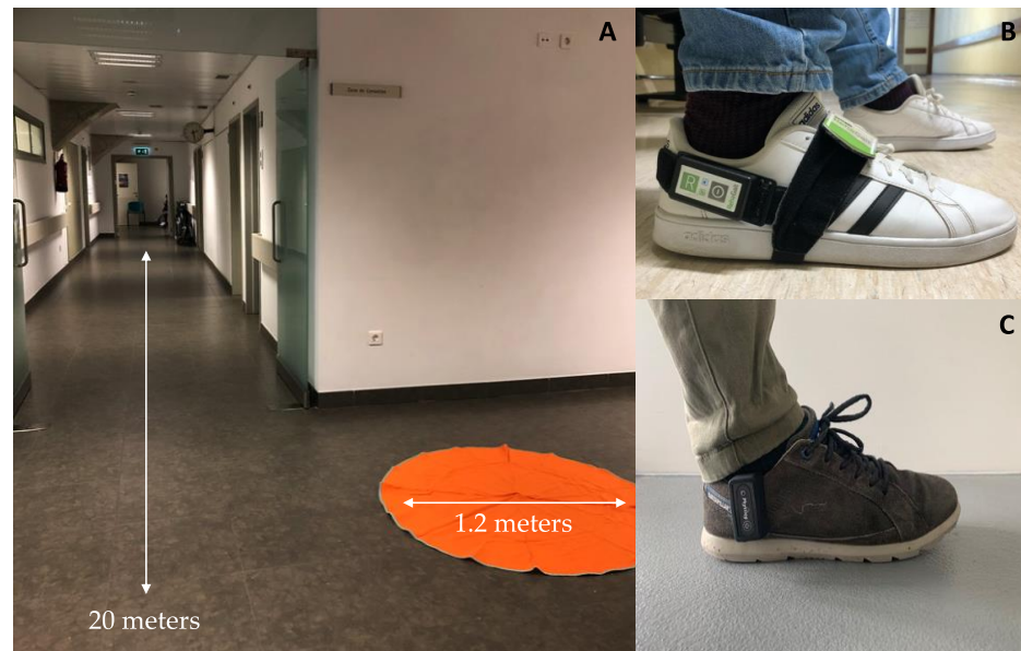
Figure 1. (A) Lab setting for the supervised assessment: 20 m walking and circular walking tasks. (B). Sensor positioning for lab assessment. (C). Sensor positioning for unsupervised assessment.
