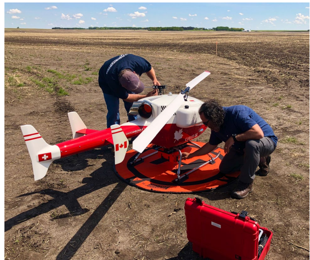
Fig. 1 SDO-50V2 multi-purpose single-engine unmanned Helicopter system equipped with the RPAS Delivered Remotely TeleMentored Self-Diagnostic Ultrasound System being prepped for take-off
