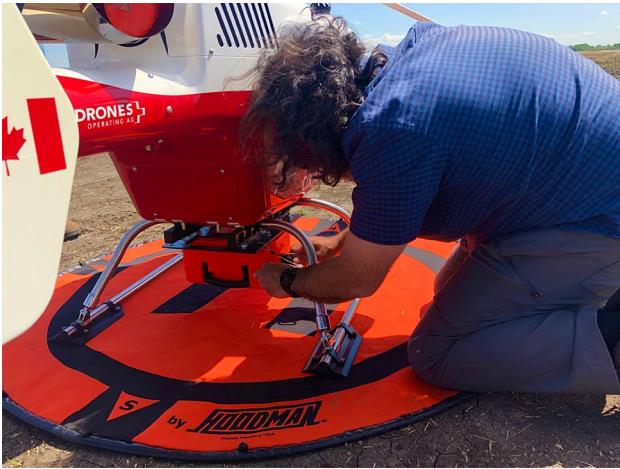
Fig. 3 Location of the RPAS Delivered Remotely TeleMentored Self-Diagnostic Ultrasound System under the SDO-50V2 multi-purpose single-engine unmanned helicopter
