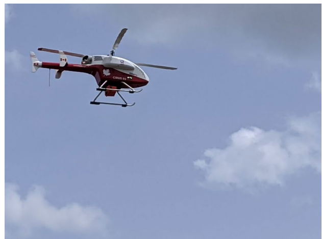
Fig. 2 SDO-50V2 multi-purpose single-engine unmanned Helicopter system equipped with the RPAS Delivered Remotely TeleMentored Self-Diagnostic Ultrasound System in flight
