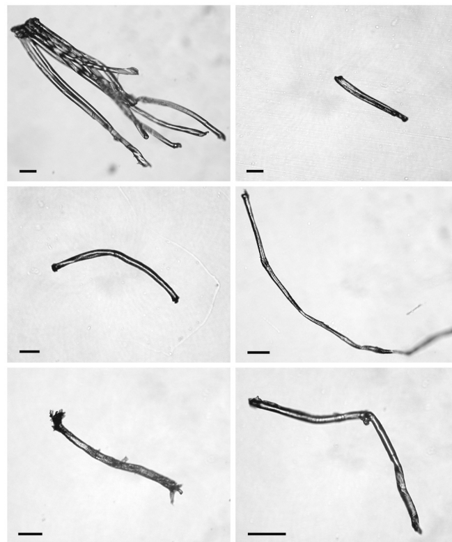
Fig. 2. Selected images of microplastic fragments and fibers excised from the PP filament web of the face mask fabric and released in water during the shear tests (scale bar = 0.1 mm).
