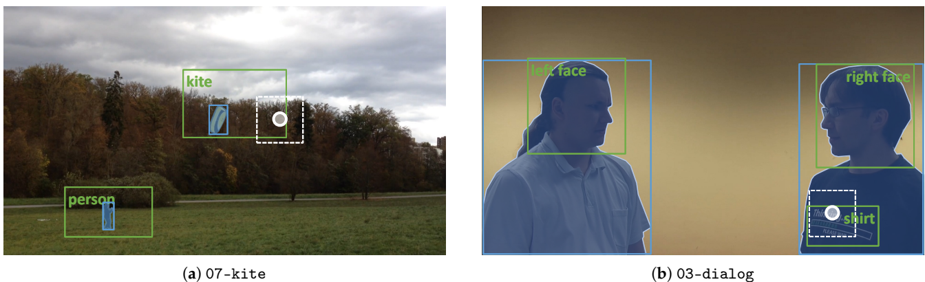
Figure 7. Example frames from two scenarios of the VISUS dataset [2] showing the recent fixation (white circle), ground truth annotations (green), object masks and bounding boxes for OD (blue), and the cropping area for IC (white rectangle).
