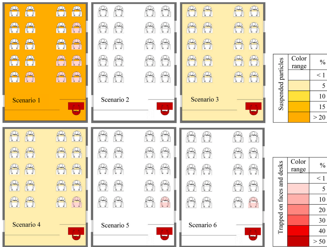
Fig. 20. Contours of fraction deposited particles on surfaces with high-level risk (faces and desks) and suspending particles in air for first six scenarios in state A.
