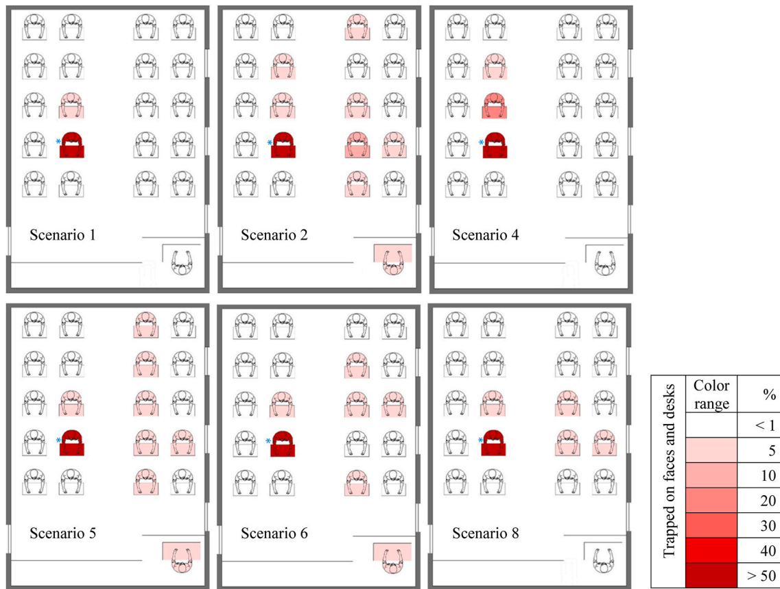
Fig. 22. Contours of fraction deposited particles on danger surfaces (faces and desks) for scenarios with high-level risk when cough source is student 7.
