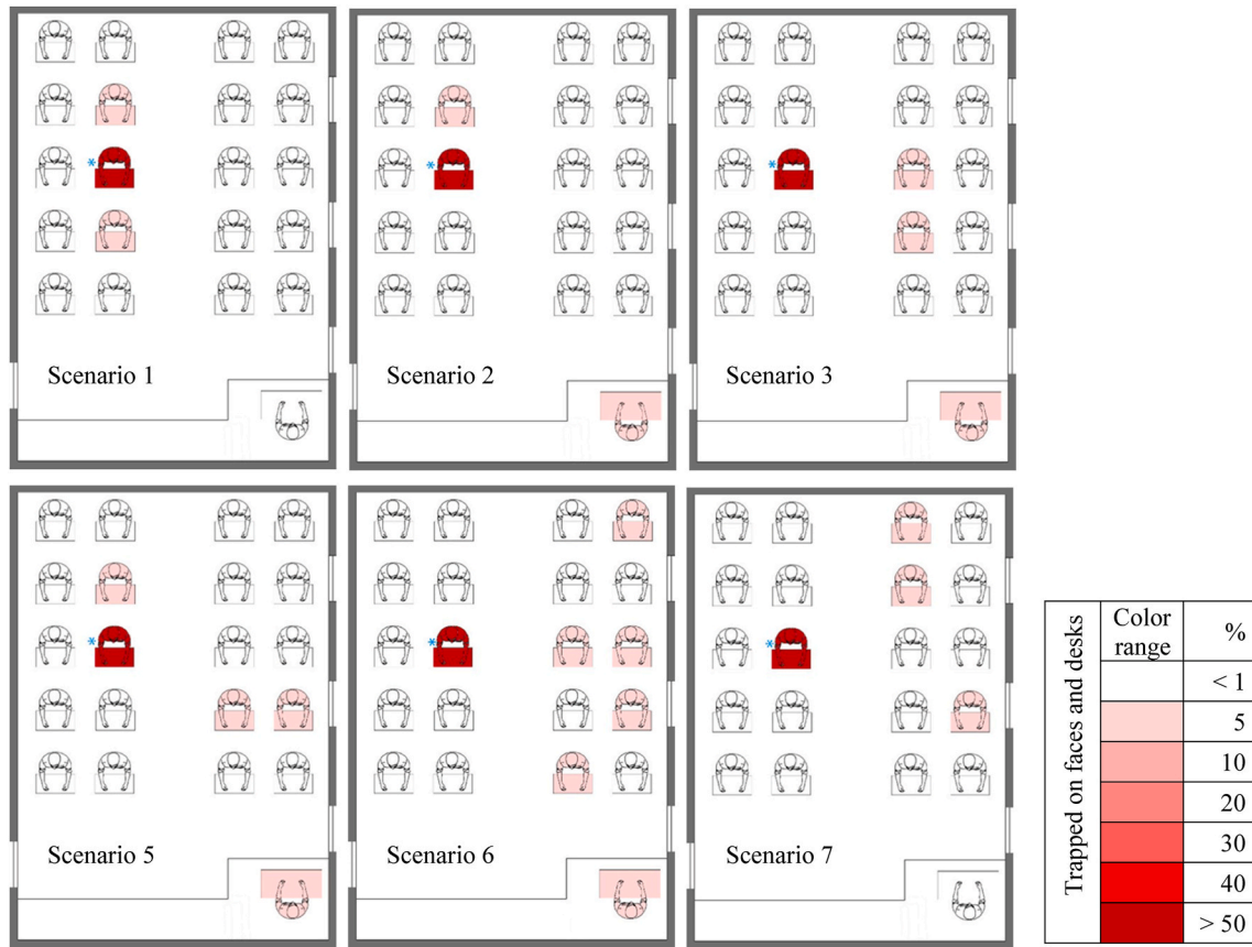
Fig. 24. Contours of fraction deposited particles on danger surfaces (faces and desks) for scenarios with high-level risk when cough source is student 11.
