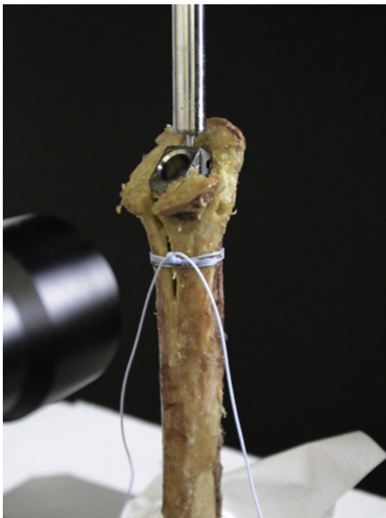
Figure 1 Suture cerclage fixation using FiberWire 5.0. Picture with reprint permission Elsevier (License 4960740921461) from Renner N et al ( https://doi.org/10.1016/j.jse.2014.02.012 ).
