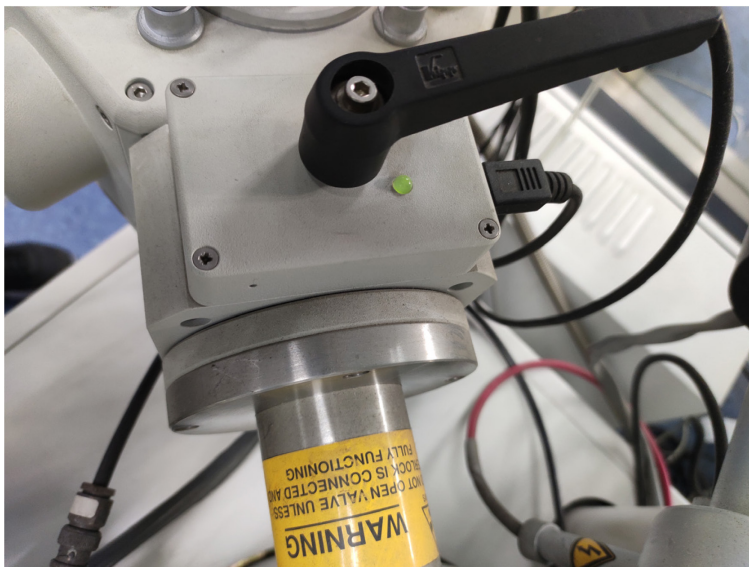
Figure 11. The ball valve LED is green. When the vacuum in the prep chamber and the SEM equilibrates, the LED turns green, and the mechanical interlock can be opened.
