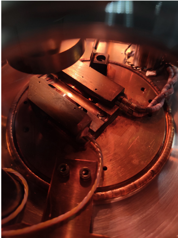
Figure 5. The dovetail stage in the prep-chamber. The dovetail stage is convenient for the angled sides of the sample holders and is fitted with a thermometer and a heater. There is a stopper to allow the sample holder to be transferred to exactly the same position. A spring clip secures the holder and prevents vibration.
