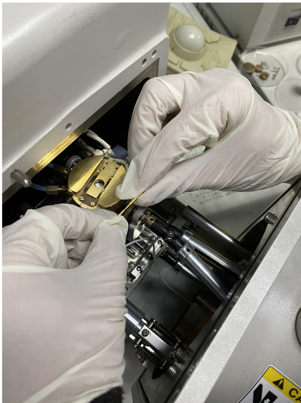
Figure 1. SEM stage cold module installation. Dovetail and fit the module with a thermometer. Push the copper shaft and copper shaft sleeve together to make an interference fit connection. Ensure that the real-time module temperatures are displayed on the keypad.
