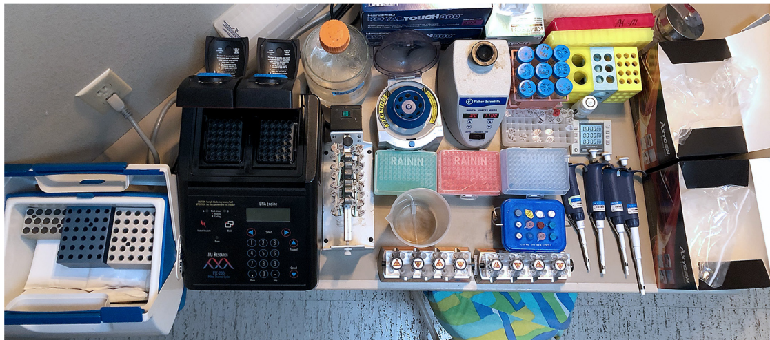
Figure 1. A home workbench for CUT&Tag. Photo of the home workbench setup used for all experiments presented using this protocol. A typical experiment begins by mixing cells with activated ConA beads in up to 32 single PCR tubes, with all liquid changes performed on the magnet stand. The only tube transfer is the removal of the purified sequencing-ready libraries from the SPRI beads to fresh tubes for TapeStation analysis and DNA sequencing. The total time from thawing frozen nuclei until elution from SPRI beads is ~8 h.
