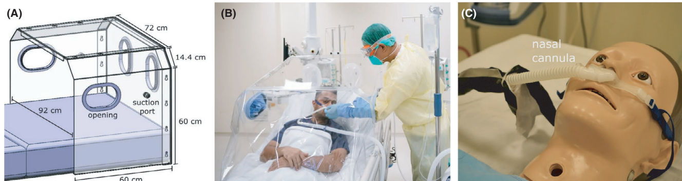
FIGURE 1 A, Barrier enclosure design used to contain aerosols from (B) patients who typically require supplementary oxygen treatment (C) delivered through a nasal cannula
