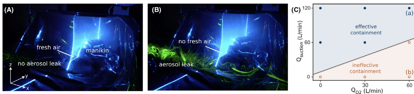
FIGURE 4 A, Aerosol is effectively contained when Q_{\text{suction}} > Q_{\text{O}_2} + Q_{\text{air}} . B, Otherwise, aerosol leakage from the enclosure can be readily observed. C, Phase diagram for effective (blue filled dots) and ineffective aerosol containment (unfilled red dots)
