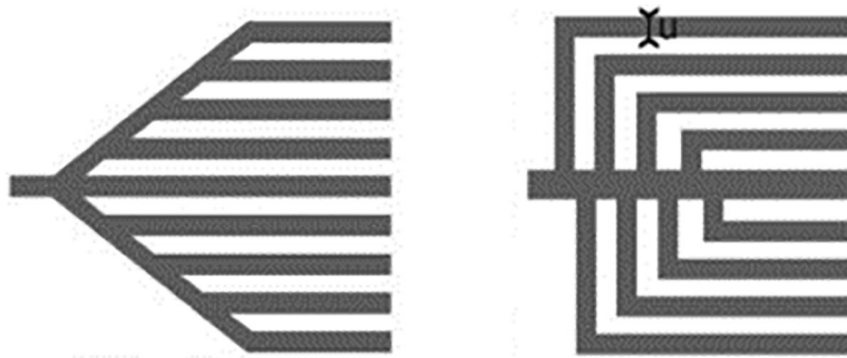
Figure 1. Tree-line capillary pump designs from Zimmermann et al. 12
