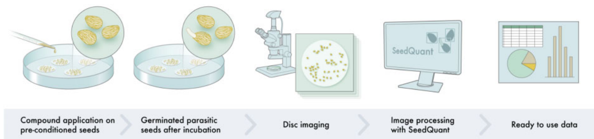
Figure 5 Proposed workflow for seed germination stimulants/inhibitors studies using SeedQuant. Stimulants or inhibitors are applied to preconditioned seeds, placed on small (9 mm) glass fiber filter paper disks. After incubation, the disks are imaged under a binocular microscope mounted by a charge-coupled device (CCD) camera. In one click, the resulting pictures are processed by SeedQuant, which renders the germination ratio for each picture. The data are then provided to the user in an easy-to-use format (.csv), allowing further data processing.
