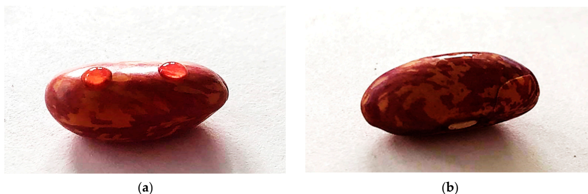
Figure 2. Water droplets on the surface of (a) an untreated bean seed and (b) a bean seed treated by plasma at t = 3 s, p = 10 Pa.
