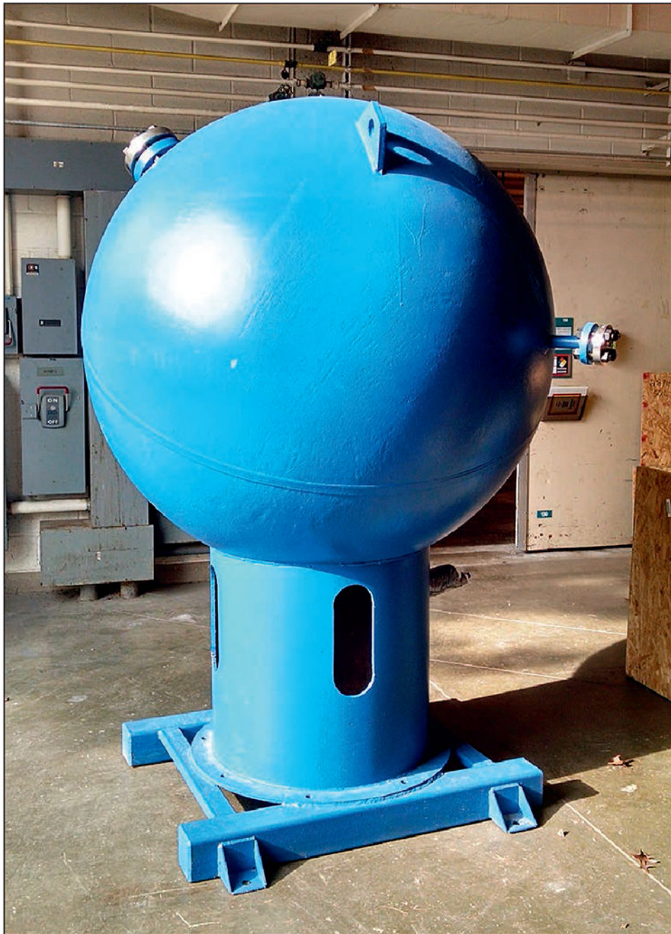
Fig. 1. The Big Blue Ball. It is made of carbon steel, has an inner volume of about 1800 liters, and weighs more than 1000 kg. (photo credit: NIST's Fluid Metrology Group).
