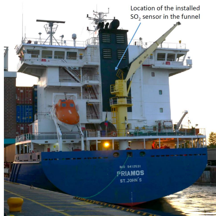
Figure 8. The container ship PRIAMOS with the approximate location of the installed and newly developed photoacoustic SO 2 sensor.
