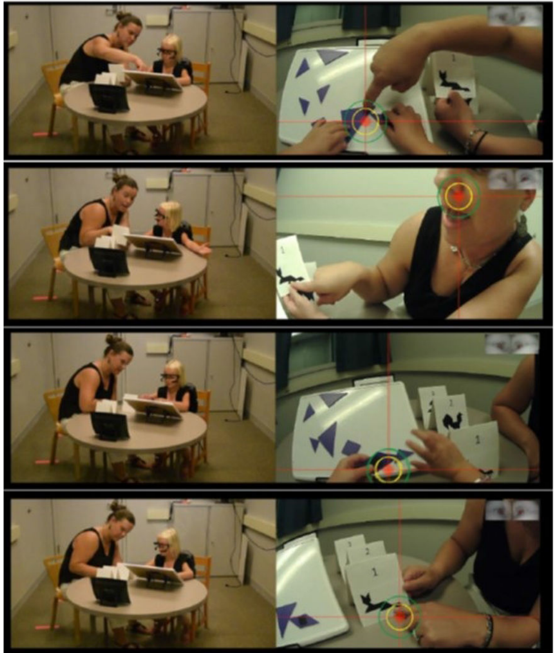
Figure 1. Example of a parent-child dyad during the PCCT. Room camera is on the left and eye tracking world camera is on the right.
