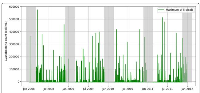
**Fig. 3** Estimates of cyanobacteria concentrations at the Wachusett drinking water intake during 2008–2011. Cyanobacteria concentrations were calculated as the maximum value of the five satellite pixels within a 900 m buffer of the drinking water intake. The shadowed data in December, January and February were not used in the statistical analysis
