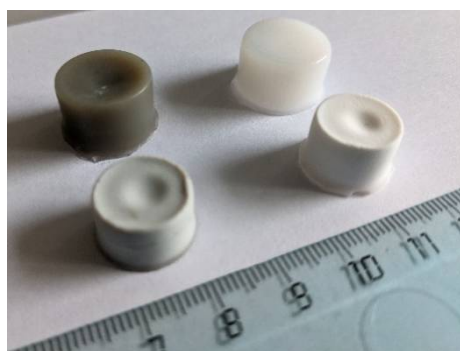
Figure 2. Digital photo of the prepared cellulose hydrogels (top row) and aerogels (bottom row).
