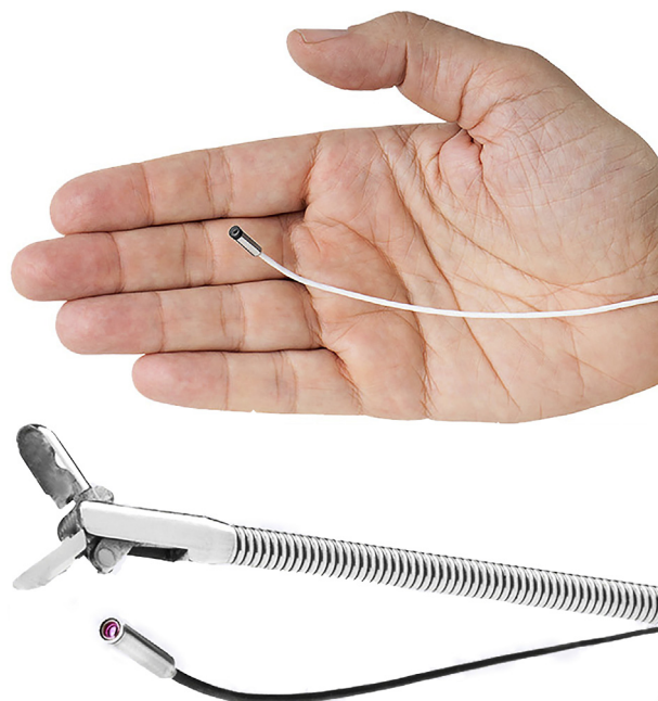
FIGURE 1. Miniature cameras (3 mm top, 1.2 mm bottom) designed for medical applications. The author was granted permission by ScoutCam to use images from their Web site ( www.scoutcam.com ) for academic publications. 3
