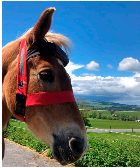
Figure 1. The wearable horse unit of the automated equine monitoring system (Hoofstep ® ) is attached to the horses' forehead using a special flexible softshell head collar.
