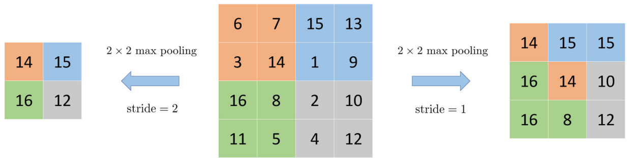
Fig 5: A 2 \times 2 max pooling layer extracts the maximum of 2 by 2 neighboring pixels / features across the spatial dimension.
