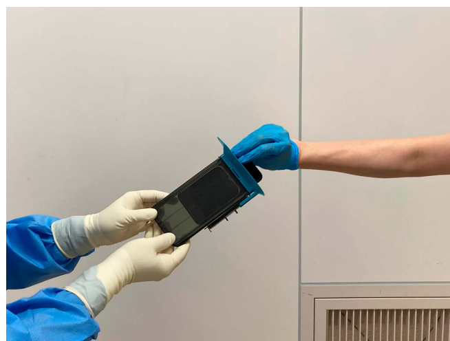
Fig. 6 Sterile smartphone cover to manage sterility in the operative field. The nonsterile mobile device is inserted into the sterile smartphone cover (CleanCase; SteriDev). The surgeon can operate the smartphone with gloved hands.
