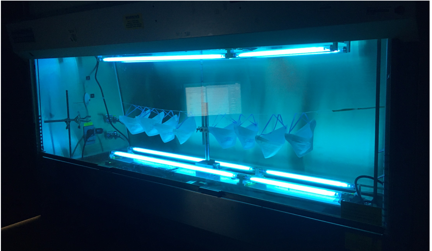
Fig 4. UVGI decontamination chamber constructed within a modified cell culture biosafety hood. Two identical four-bulb UV-C arrays were placed facing each other within the hood, and were used to decontaminate masks prior to construction of the larger array (Fig 1).
