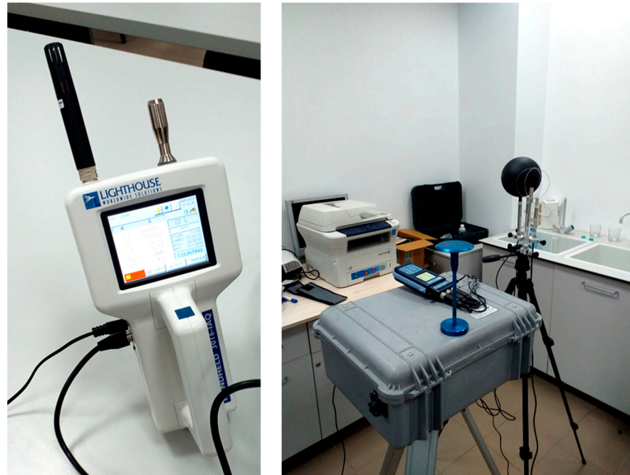
Figure A1. Instrumentation used in the current study (particle counter, PM monitor, and thermal microclimate equipment).
