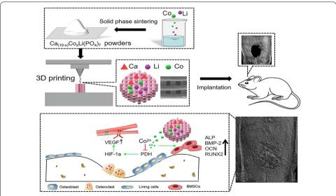
**Fig. 1** Schematic illustration of the fabrication of porous bioceramic scaffolds doped with different amounts of cobalt to promote bone defect repair via enhanced osteogenic and angiogenic properties
