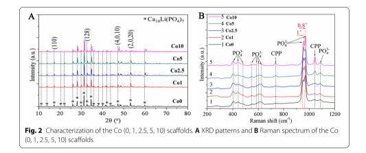
Figure 2B displays the Raman spectra of the Co (1, 2.5, 5, 10) scaffolds. Compared with the Co0 scaffold, the band positions of the Co (1, 2.5, 5, 10) scaffolds were altered, moving to the direction of a higher Raman shift with increasing Co-doping level.
