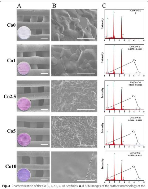
Co (0, 1, 2.5, 5, 10) scaffolds with EDS analysis (**C**) (scale bars: Figure  $\mathbf{A} = 500 \, \mu \text{m}$ , Figure  $\mathbf{B} = 10 \, \mu \text{m}$ )
