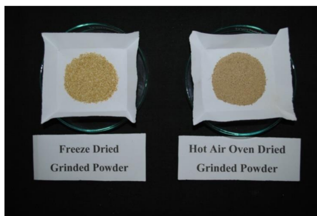
Figure 6. Freeze dried and hot air oven dried grinded powder of physiologically dropped immature mandarin ( Citrus reticulata Blanco) fruits.
