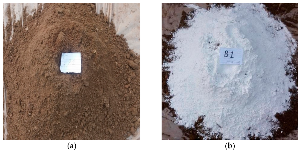
Figure 1. View of: (a) clay sample, and (b) mixing of clay and marble dust.
