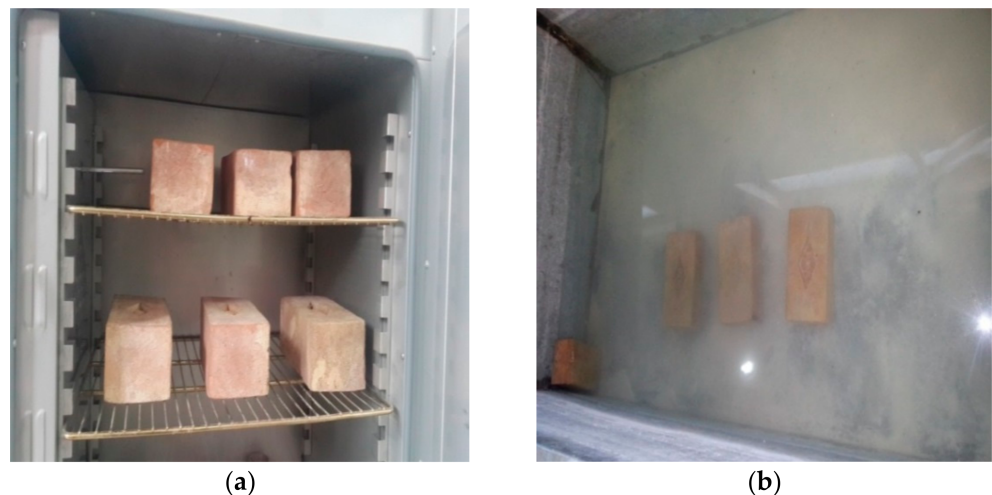
Figure 4. Water absorption test: (a) drying the samples in the oven, and (b) soaking the samples in water.
