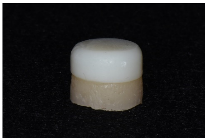
Figure 2. Specimens used in the experiment (Top: LiSi Press, Bottom: Charmfil flow).
