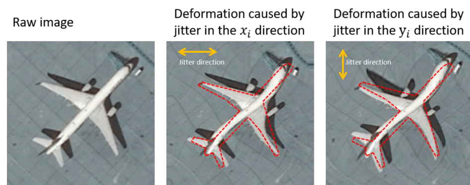
Figure 2. Image deformation caused by jitter in the x_i and y_i directions.
