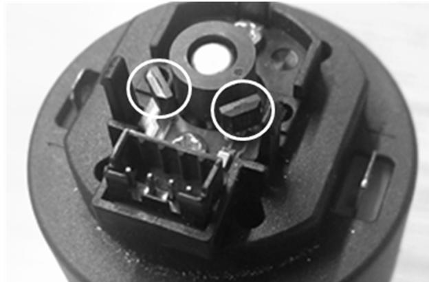
**Figure 2.** Detail of the low-cost magnetic encoder showing the magnetic ring attached to the motor shaft and the two Hall-Effect sensors (white circle).
