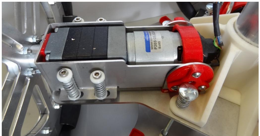
**Figure 1.** Detail of the compact motorization P205-2S.12.64 that includes a brushed DC motor, a 1:64 gear (at the front), and a six-pole low-cost magnetic encoder (at the back).
