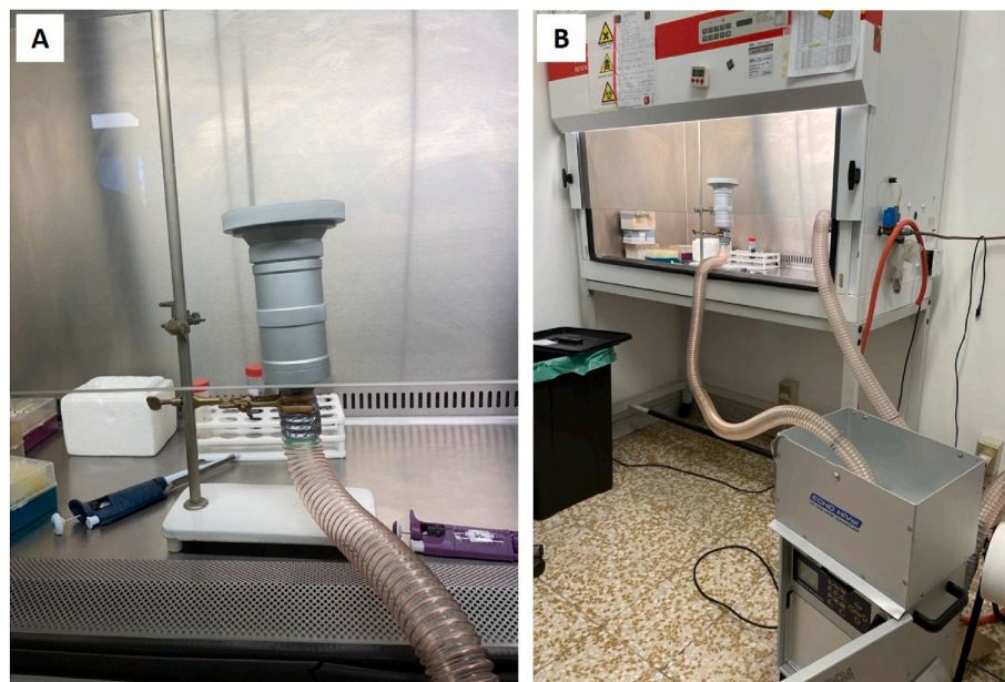
Fig. 1. Experimental setting for recovery tests with aspiration in biosafety level 2 (BSL-2) conditions. A fixed inoculum of HCoV-OC43 suspension (50 µl) was spotted on glass-fiber filters of 10 cm diameter and placed on a sampling head (A), and a high-volume sampler for air filtration was used (B).
