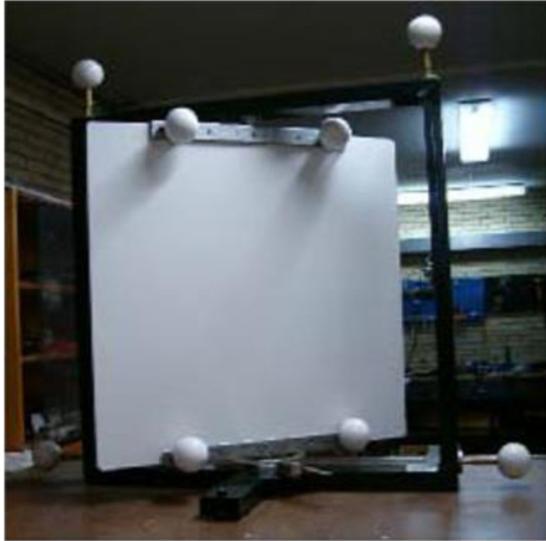
Fig. 25. Artifact to estimate effect of angle of incidence. Reproduced from Kersten et al [134].
