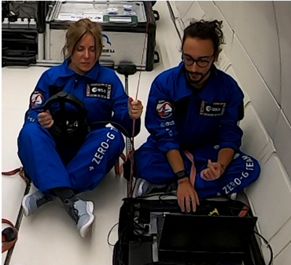
Fig. 4 Photo of the experimental set-up in flight. The participant was sitting cross-legged and firmly strapped to the floor at 60 cm from the screen of a laptop that was attached on the floor and centred on the sagittal mid-plane. The experimenter in charge of administering the experimental task and supervising its execution was positioned on the right side of the participant, slightly further back so as not to interfere with task execution.
