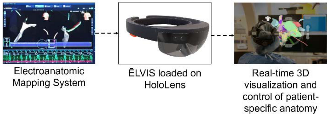
Figure 4. Workflow for the Enhanced Electrophysiologic Visualization and Interaction System, or ELVIS. Data flows from the electroanatomic mapping system to the ELVIS application which runs off a Microsoft HoloLens. From here, the real-time patient specific data is displayed in true 3-dimensions for the physician to visualize and interact with to best understand the data during the procedure to optimize patient outcome.
