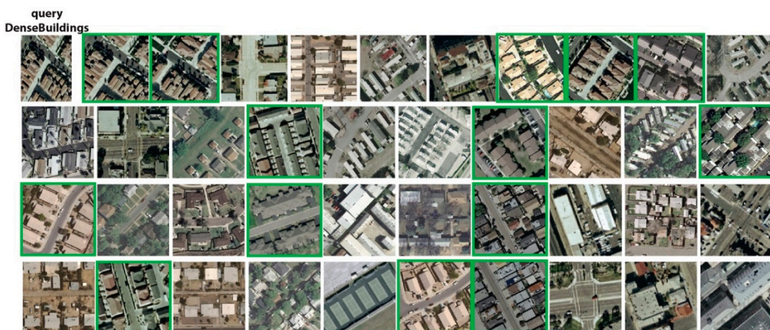
Figure 11. Retrieval results of dense-building category using convolutional neural network as a feature extractor (RL-CNN). The green rectangles indicate correct retrieval results.
