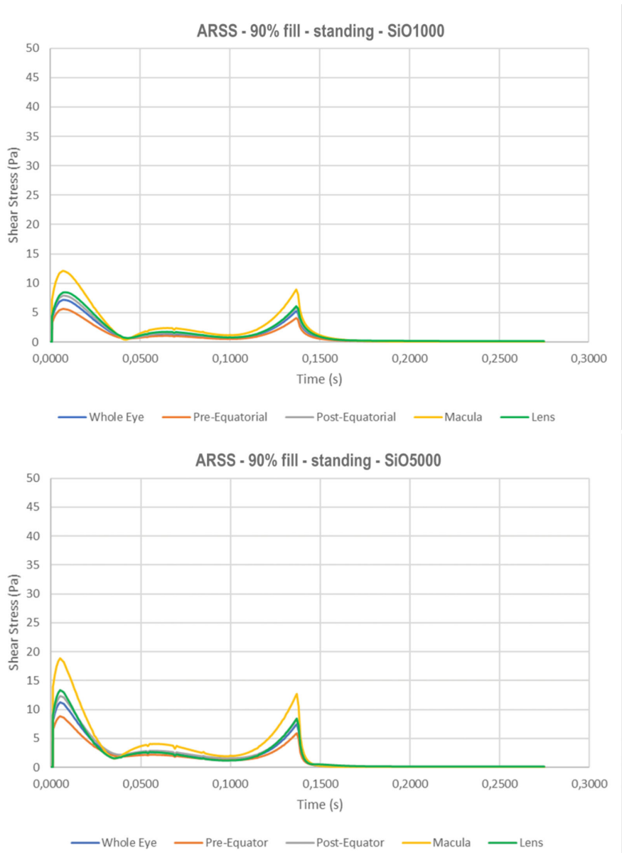
Figure 10. Average regional shear stress (ARSS) as a function of time for 90% tamponade fill. The macula is exposed to the highest mean shear stress throughout the saccade while all other sectors show significantly lower peak values: a) standing with SiO1000; b) standing with SiO5000; c) 45° tilt upward head with SiO1000; and d) supine with SiO1000.
