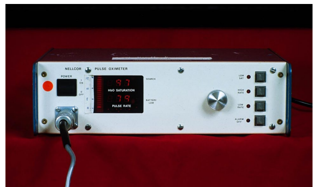
Fig. 9 Nellcor Pulse Oximeter Prototype as delivered to us in 1982. Note the absence of the "N-100" designation, this was added at a later date as N-100A. The first commercial model was called N-100B.
