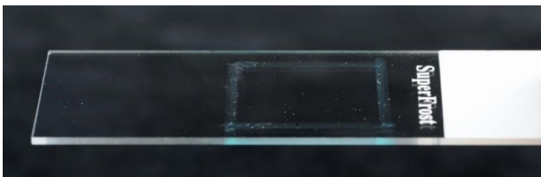
Figure 2. The surface of a glass slide showing the enclosure drawn on using a PAP pen, allowing containment of molten agarose medium
